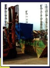
1. Driver positions Burro so that push arm on base touches edge of skip. As fork truck is driven forwards, base of Burro slides back.
