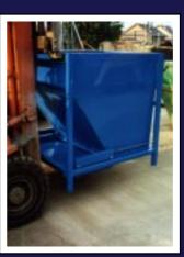
3. Empty Burro is lowered to ground level where base panel closes automatically.
