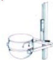
Bracket for swivelling bowls used in mixers
