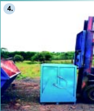
4. SUPER-BURRO is moved away from the skip and lowered to ground level where the base closes and locks automatically. There are no chains or fixings to remove.
