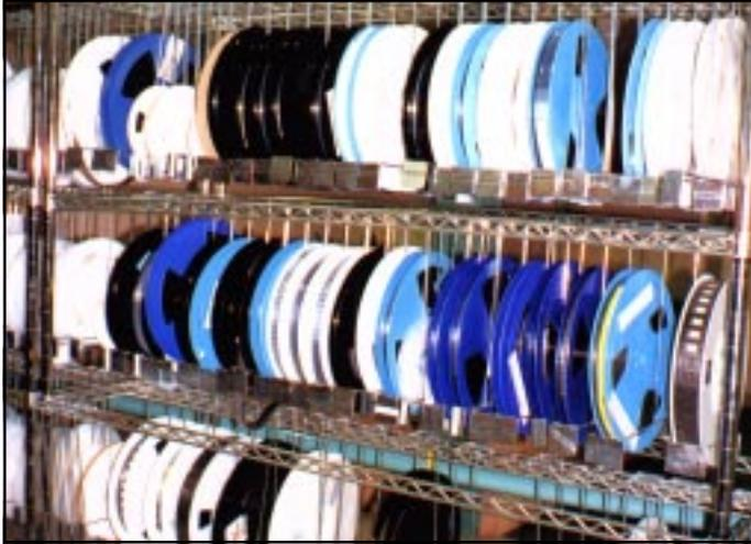
*Surface Mount Reels are easily identified and picked from either side*
